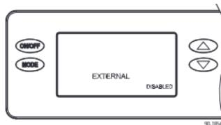
If using the dehumidifier on-board control, leave DISABLED and press MODE to go to the next screen.
