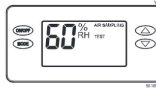
Press and hold the ON/OFF button and MODE buttons for 3 seconds. The measured humidity, AIR SAMPLING and TEST will show on the display.
