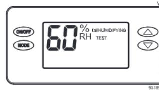
After three (3) minutes the dehumidifier compressor will turn on and DEHUMIDIFYING will replace AIR SAMPLING on the control screen.
