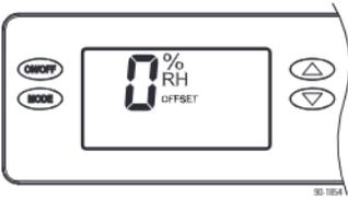
An offset can be applied to the on-board humidity reading to avoid discrepancies with other humidity measuring devices in the room. Use the UP or DOWN button to select an offset from -5% to 5%. Press MODE to exit the installer set-up screens.
