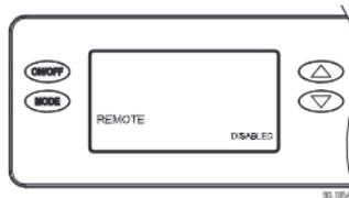
If not installing an A77, leave DISABLED and press MODE to go to the next screen..
