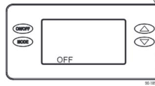
If the dehumidifier is not already OFF, press the ON/OFF button to turn it off.
