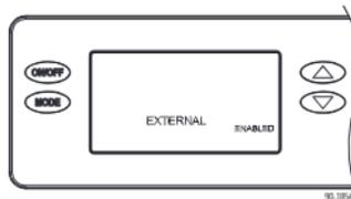
If using a Model 8800 series thermostat or alternate control as an external control, use the UP or DOWN button to select ENABLED, then press MODE to go to the next screen.
