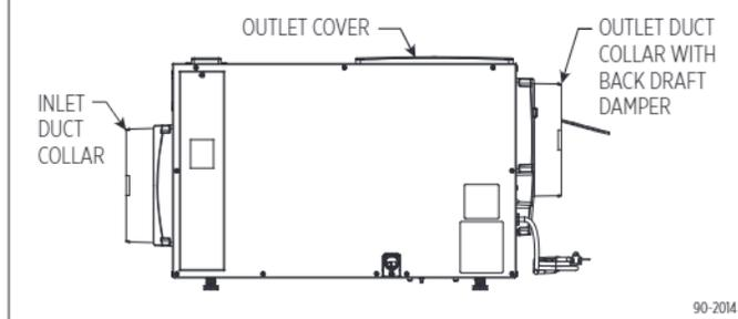
**FIGURE 3 – FLOOR MOUNT INSTALL**
