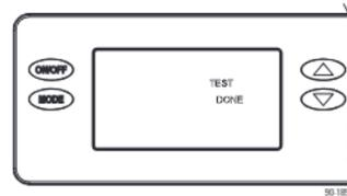
After one minute of compressor operation, all outputs will turn off and DONE will blink for 3 seconds and then return to the OFF screen.
