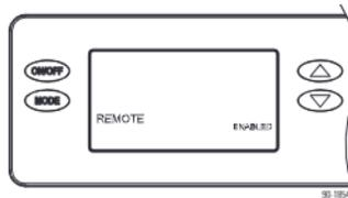
If installing an A77, use the UP or DOWN button to select ENABLED, then press MODE to go to the next screen.
