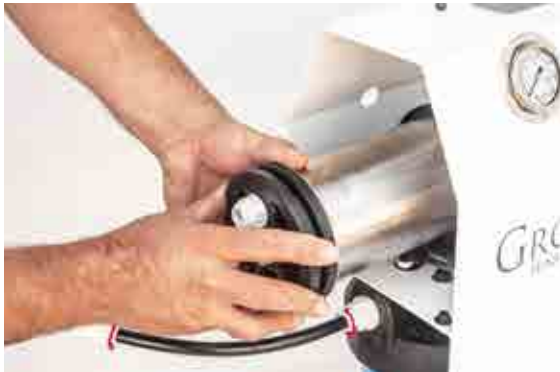
Seat the end-cap back into the input side of the membrane housing.
