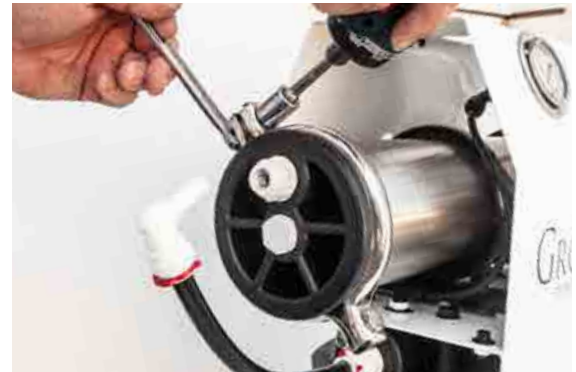
Replace the stainless clamp on the input side of the membrane housing.
