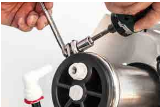
Tighten the stainless clamp retaining bolts evenly.
