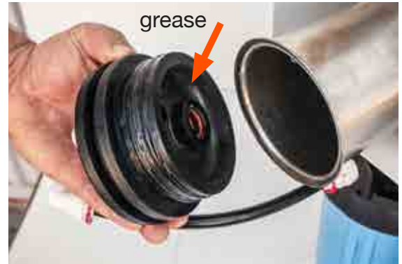
Grease the brine seal and end-cap center hole with food grade silicone grease.
