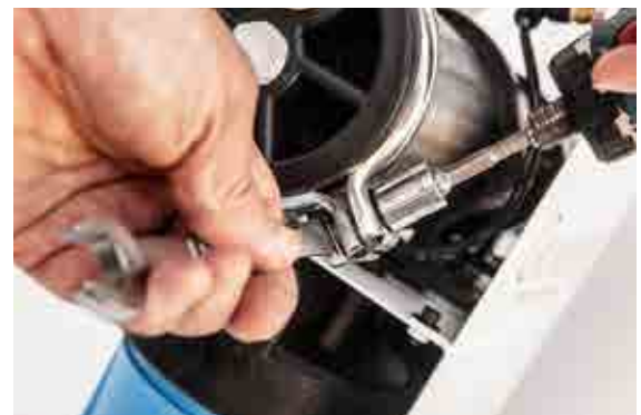
Tighten the stainless clamp retaining bolts evenly.
