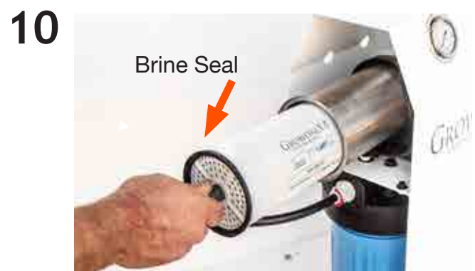
Insert the membrane element into membrane housing, making sure that the brine seal goes in last.
