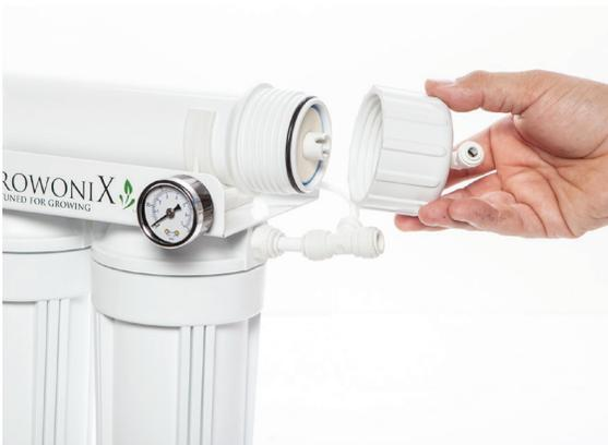
Unscrew membrane housing end cap. Caps can be difficult to remove. Be sure to have a firm grip on opposite side of housing. Do not lose O-ring on inside of cap. Each cap has two O-rings.
