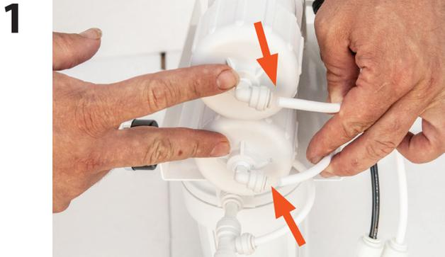
Make sure incoming feed water is shut off, ensuring the RO filter is depressurized.
