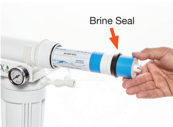
Insert new membrane into housing, making sure the membrane-end with the brine seal goes in last. Make sure membrane is completely seated in the housing.
