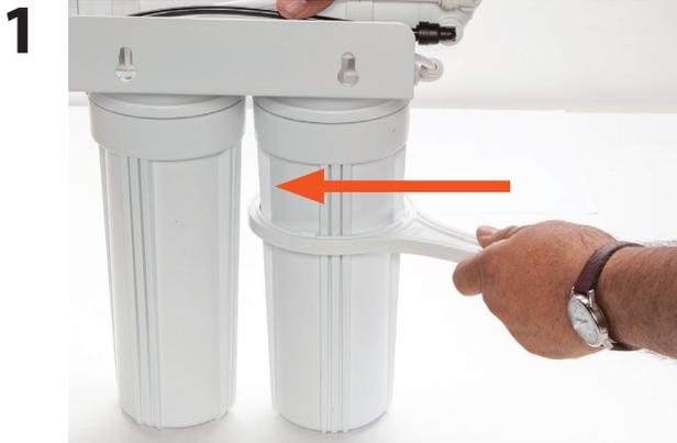
Unscrew sediment and carbon filter housings using supplied filter wrench. Wash inside of filter housings to remove debris.
