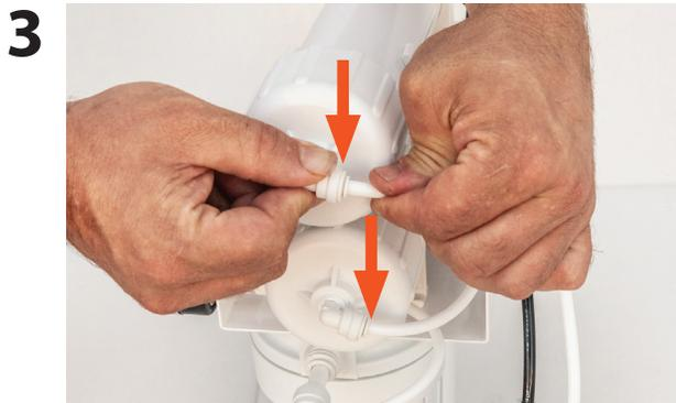
Reconnect tubing to membrane input and resume normal filter operation.
