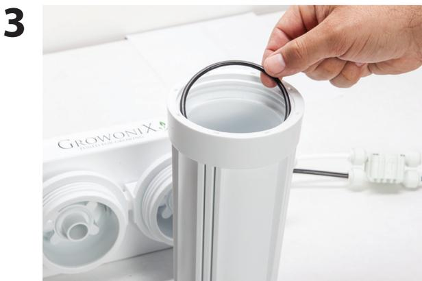
When replacing filter housings, make sure housing O-rings are seated properly. O-rings function best when lubricated with food grade silicone lubricant.
