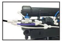
Once the initial flush is complete turn the blue valve to the closed position (perpendicular to the tubing)
