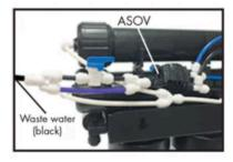
Push short piece of pre-installed black tubing on the flow restrictor/ flush kit assembly into the black quick connect fitting on the ASOV (where "out" is imprinted on ASOV)
