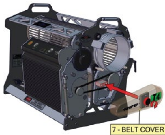
Figure 4: Installing the belt cover
