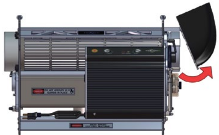
Figure 22: Removing the hopper
