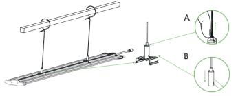
To shorten cable: Press the cable down through the cylindrical lock. (Figure A) To extend cable: Press metal top down and pull up on cable. (Figure B)
