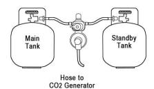
This handy valve will keep you from running out of fuel and interrupting CO2 enrichment. When fuel is depleted in main tank the valve switches to the alternate tank and indicator shows red. Disconnect spent tank and refill at your convenience.
